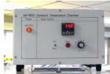
Temperature Control at 55°C in the Chamber
