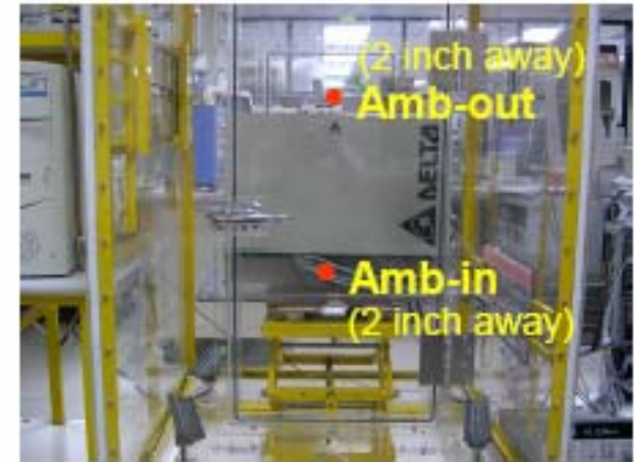
PSU in Free Convection Chamber with a Cover (@ 55°C amb.)
