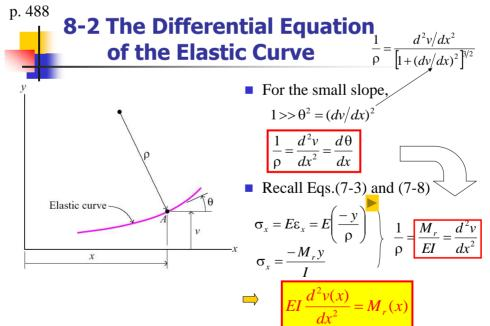
Differential equation for the elastic curve
